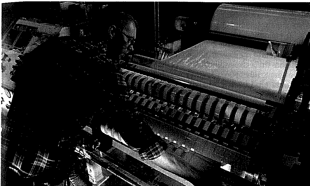
Slitting tape is now a more efficient operation at 3M's tape factory. By moving the tape coating and slitting machines next to each other and giving the operators responsibility in quality control, the factory has been able to coordinate output and cut down on both inventory and manufacturing time.
